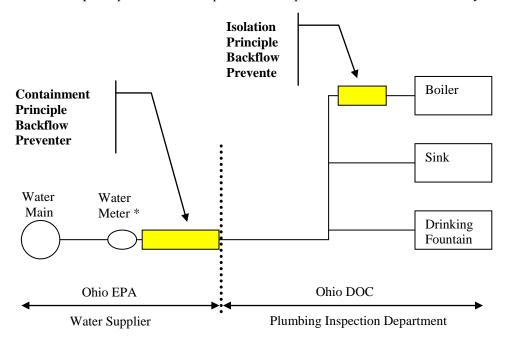
• If the water meter is installed inside the building then the containment principle backflow preventer must be installed immediately after the water meter. If the meter is installed outside the building then the containment principle backflow preventer is typically installed inside the building wall unless otherwise approved by the water supplier.
