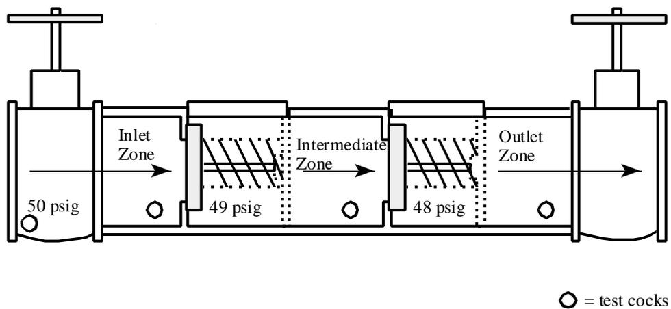
1. Under flow conditions, both checks should be open.
