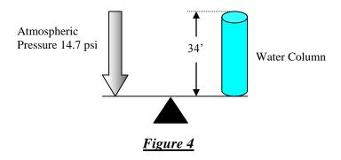
The balancing of forces is also shown in Figure 5. When a long tube closed at one end is filled with water and inverted in an open container of water, the water level in the tube will be higher than the water level in the open container. The weight of the atmosphere pressing down on the water surface in the container will hold the water in the tube up to a maximum elevation of 34 feet. One pound per square inch of pressure will elevate water to a height of 2.31 feet.
