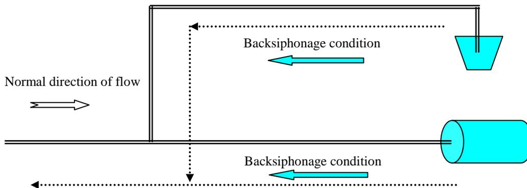
A drop in the supply pressure in the water main or in the consumer's internal piping will cause a reversal of flow in the piping due to backsiphonage.
