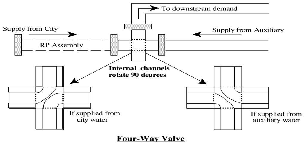
The drain port on the four way valve shall not be installed in the vertical position
